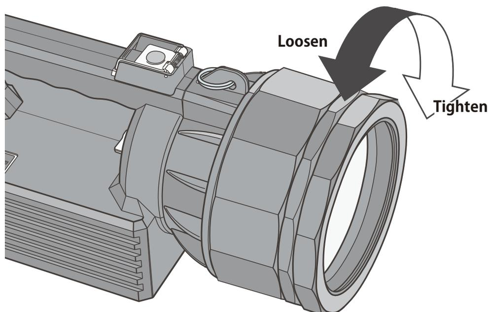
(1) Remove the lens cover by turning in anti-clockwise direction.
